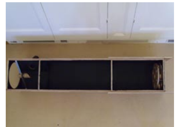
Paint the inside of the tube matt black, plus side four
