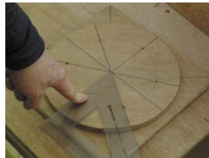
Divide the mirror cell, a round from a baffle, into thirds
