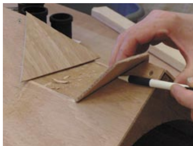
Mark up two 3mm triangles for the sides of the rebate
