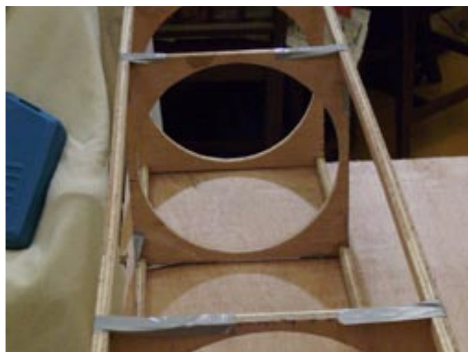
Tape the joints up to make sure the glue bonds well
