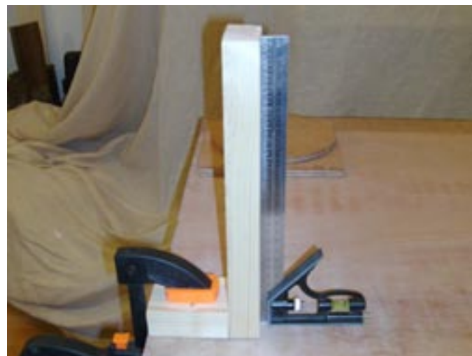
A support helps you glue the skeleton together square
