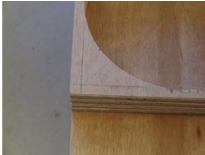
Mark the baffles with 12mm square indents for the struts
