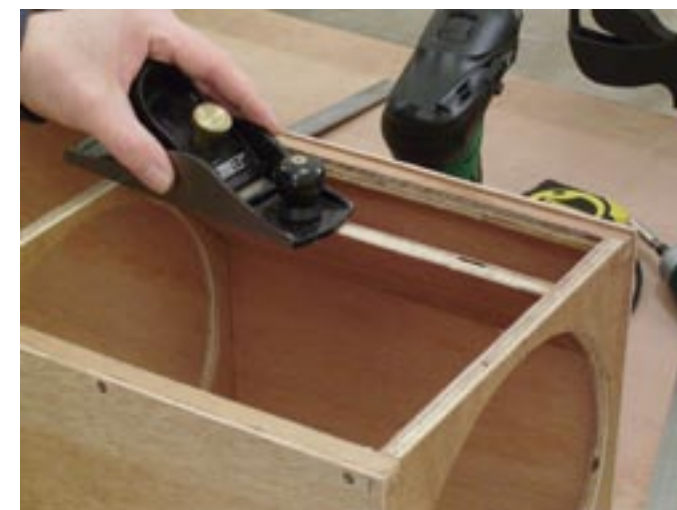
Use a plane to make sure all surfaces are flush
