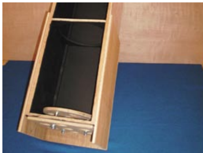
Attach the 9mm plywood, overhanging the base by 60mm
