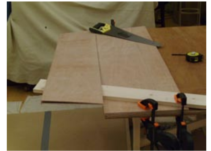
Now cut out the skin from the 9mm plywood sheet
