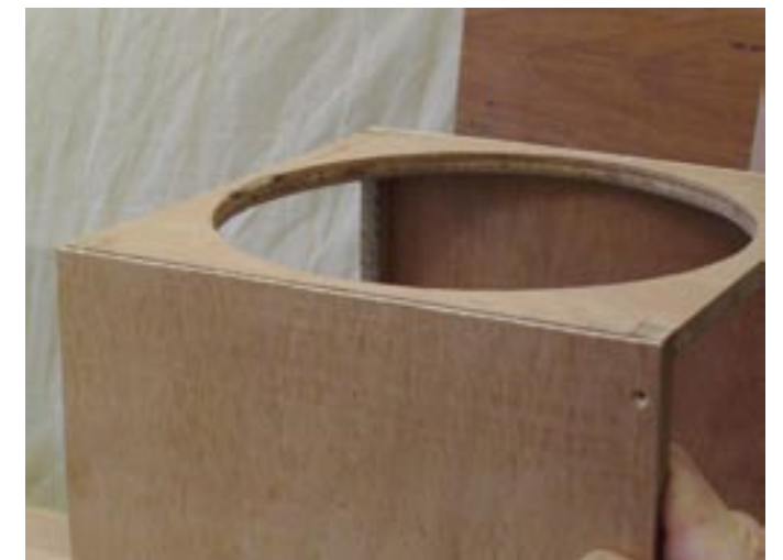
The skin should be flush with the top and bottom baffle
