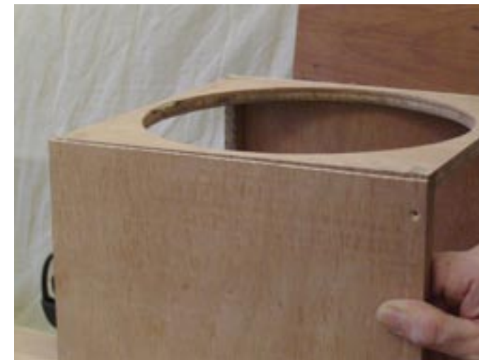
The incorrect way of lining the skin up with the baffle
