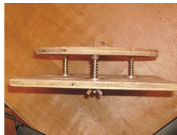
Between the cell and backplate are three sprung bolts
