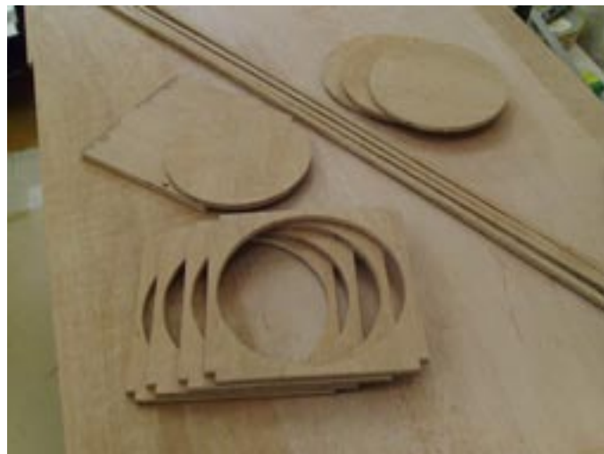
Struts, baffles, mirror cell and rounds from the 12mm ply
